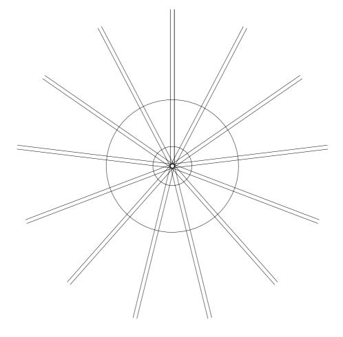
The actual width of each slot should be approx 4 x the diameter of the wire used.
